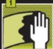
Clean and degrease surface. Abrade the surface with P80-P120 grit sand paper. Reclean.
