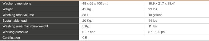
Designed to clean automatically spray guns and painting accessories when working with solvent-based paints and clearcoats.
