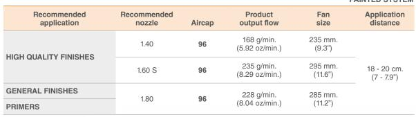
Air consumption at 2 bar (29 psi): 280 L/min. (9.88 cfm)
